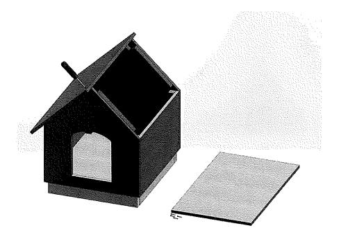
To keep the dog house dry, you can cover the entire roof with tar paper fastened with staples. Once you've covered the roof, you can then add shingles.
