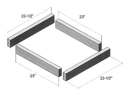
☐ Attach the base pieces together using 3" galvanized wood screws in each end
