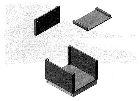
Attach the front and back panels. Place the front and back panels on the floor base and attach to the framing with galvanized wood screws every 4-5 inches around the perimeter
