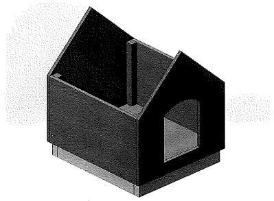
Attach the 13" 2x2 roof framing piece to the inside edges of the front and back panels halfway between the top and bottom of the angled side of each panel. Screw three 1-1/4" galvenized wood screws into each panel
