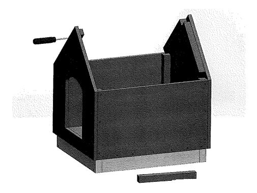
Install rigid foam insulation in the wall cavities. Use 1-1/2" thick foam, cut these to fit and then cover them with 1/4" plywood. Add 2x2 framing if required to attach plywood.
